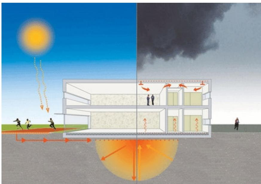
The sun beating down on the playground tarmac heats the water in the pipes of the collector. The water is pumped to the thermal store beneath the building. On cold days the heat is extracted from the thermal store and used to heat the building
